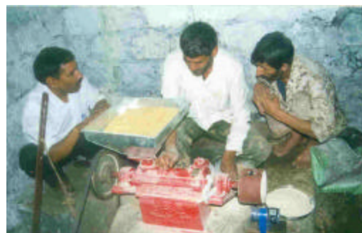
Rice Hulling with Improved Watermill Source: IT Power India
